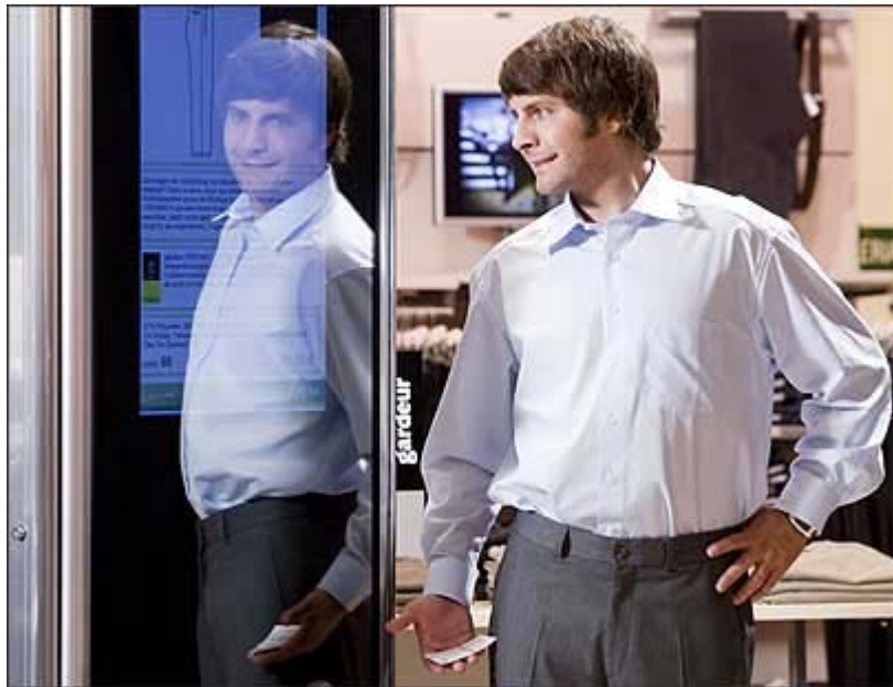
After trying on a garment, the consumer can approach a smart mirror outside the dressing room, which provides similar information to that provided in the dressing room but does not include a touch screen.
