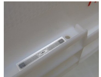
The picture shows the label to be applicated underneath the outer rim; the plastic crate is upside down.
